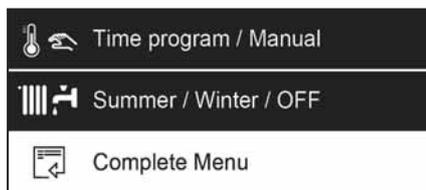
2 The “+” and “-” buttons are used to select the parameter set and make adjustments to individual parameter settings. The **OK** button selects the parameter set and confirms and stores any adjustments made.
