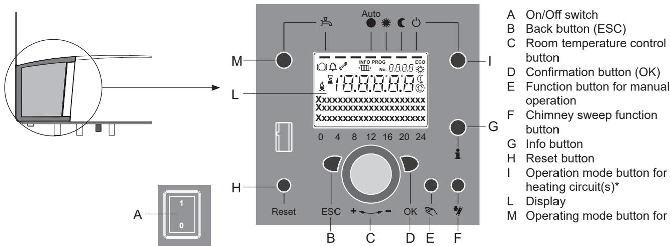
The display shows the boiler water temperature in °C as standard and the indicators under the programs that are switched on.
