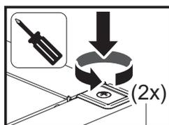
After working on the boiler always put back the cover and tighten with the 2 screws.
