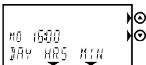
Press (DAY) and the day indicator starts flashing. Set the correct day using the arrow keys and .
