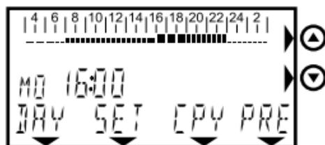
The small blocks which are no longer flashing have been set, i.e. for 7:00 to 16:00 hours inclusive T2 has been set.
