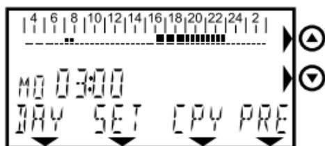
Now, using the arrow keys, you can run through the time bar without the temperature changing.
