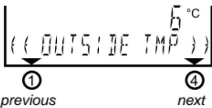
1. Outside temperature. If  $\_ \_ \_ ^\circ\text{C}$  appears on the screen, then there is no outside sensor connected or it is not working.
