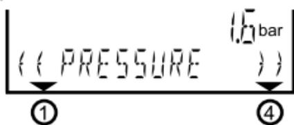
2. Pressure of central heating installation.
