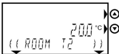
Set the required (middle) temperature T2 using the arrow keys.
