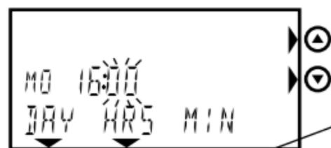
Press (MIN) and the minute's indicator starts flashing.
