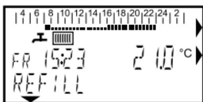
The central heating's pressure is too low. Top up the central heating system. Refer to the boiler's manual for additional explanations in this respect.
