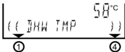
5. Hot water temperature (Not every boiler type displays this temperature)
