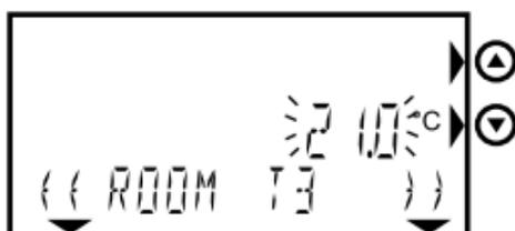
Set the required (highest) temperature T3 using the arrow keys.
