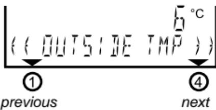
1. Outside temperature. If \_ \_ °C appears on the screen, then there is no outside sensor connected or it is not working.
