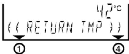
8. Central heating's return temperature inside the boiler
