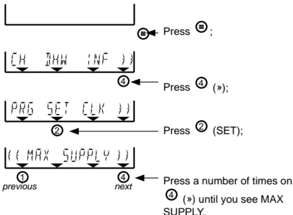
MAX SUPPLY = CH setpoint (= maximum flow temperature).
