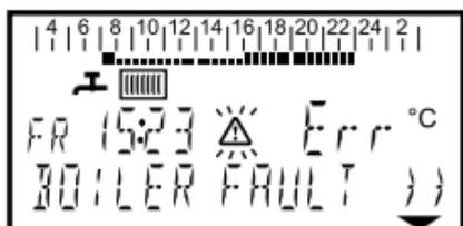
If it reads "Err" instead of the temperature then there is something wrong with the boiler's thermostat. Check whether the wiring has been properly connected to the boiler (to the Z-ready/bus-thermostat connection) and
