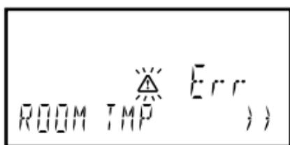
This fault implies that the thermostat is not working. The thermostat may supply some heat (central heating's input temperature  $\pm 40^{\circ}\text{C}$ ), but the thermostat needs replacing.
