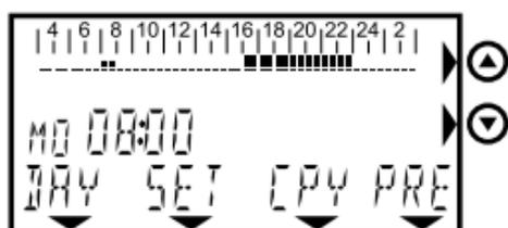
Use the ▲ key to run through the time bar until 16:00 hours appears on the screen.
