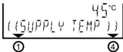
3. Central heating's input temperature inside the boiler
